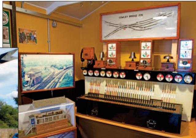
△ Elsewhere on the site there is a miniature lever frame with full size instruments which is based on the signal box at Cowley Bridge Junction, just outside Exeter. On Open Days this can often be seen being operated by volunteer signalmen.
