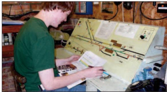
△ A simulator downstairs enables visitors to be given demonstrations of the signal box in operation. It also enables enthusiasts and professional signalmen to operate the signal box to a full timetable as if for real, without the risk of crashing any real trains.
